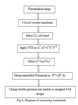
Step 3: Now by using values of U w, V<sub>w</sub> and S<sub>1</sub> \*, obtain D\* according D\*= U<sub>w</sub> S<sub>1</sub> \*V<sup>T</sup>, in the end we can obtain the watermark which is embedded according to W\* =  $(D^* - S) / \alpha$ .
